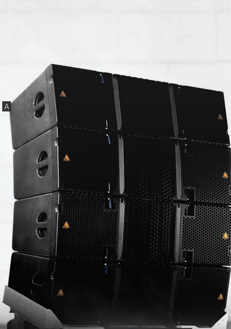
A. E12: 3-way line source enclosure: LF - 2x 12" ND12-S, MF - 1x 7" YX7, HF - 1x 4" NH4TA2, Autolock™ rigging system
